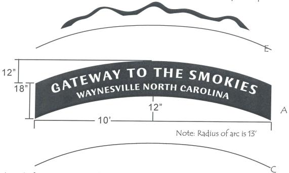
A. Identical panels, front & back. To include laser cut lettering as specified. 1/4" steel, powder coated. Panels should be assembled as single unit (Parts A, B, C, E) separate from posts. Only "D" should be permanently welded to posts. Finished project will consist of 2 identical posts and the assembled arch.
